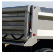
DuraClass bodies come with full depth corner posts and enclosed tailgate hardware, another premium feature you won't find anywhere else in the industry.
