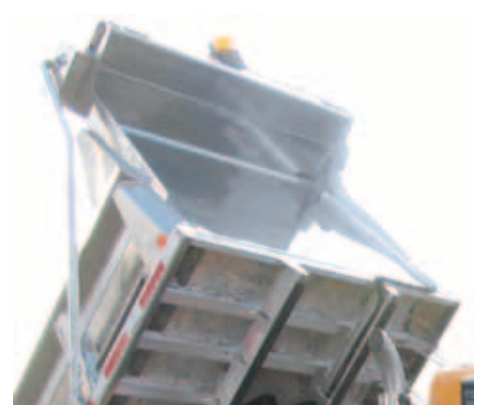
The aluminum design features a stacked understructure of 5 3/4" I-beam longmembers and 4" crossmembers on 12" centers for maximum floor support.
