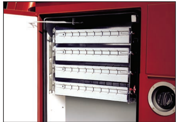
Nested slide out trays—shown closed. Available with 150 and 250 lb. capacity trays.
