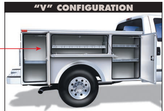
"V" Configuration with two full height vertical compartments
