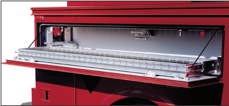
Single slide out trays available in 150 or 250 lbs. capacity. Horizontal door with heavy duty cable retainers provides a smooth, level work surface.
