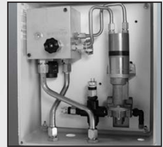
LS102H (Hydraulic Enclosure with Proportioning Valve)
