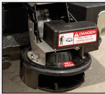
NEW high flow chute with larger 14" spinner, open trough, and shield that better protects truck from flying salt
