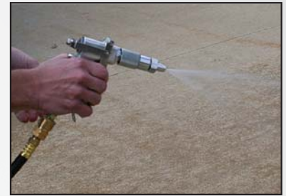
adjustable spray nozzle - pressure switch activates pump on demand
