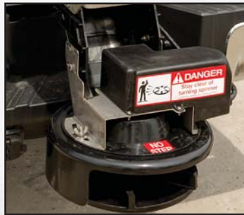
NEW high flow chute with larger 14" spinner, open trough, and shield that better protects truck from flying salt
