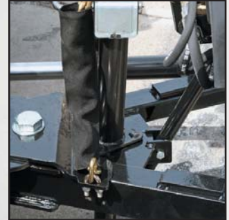
Adjustable/removable jack stand provides max. flexibility for a wide range of mounting conditions & surfaces
