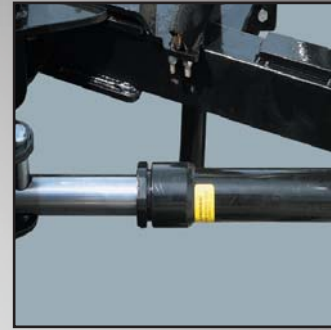
1/2" x 12" Angle cylinders provide greater angling force than standard cylinders
