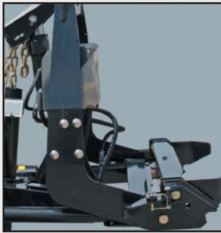
Contoured lift frame allows for greater ground clearance
