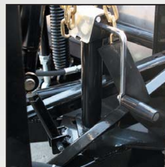
Adjustable / Removable jack stand allows for maximum flexibility for a wide range of mounting conditions and surfaces
