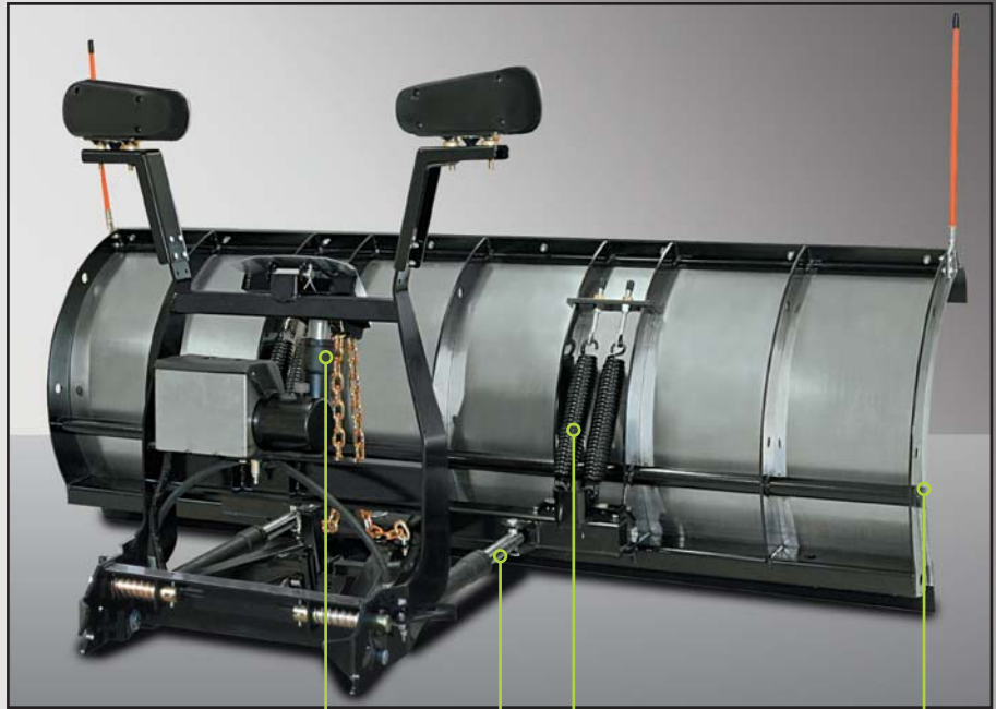
1/4" Laser cut steel ribs w/2" cross tube and HD channel, spreads loads across components, not connection points
