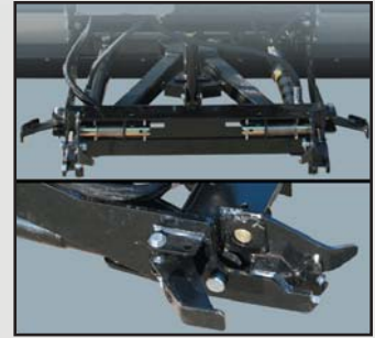
Easy to use over center linkage operated locking pins with foot pedals, allows for quick mounting & dismounting of plow
