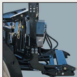
Contoured lift frame for greater ground clearance
