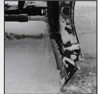
Trip edge design for smooth plowing over obstacles
