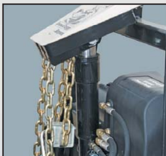
Lift arm w/heavy-duty 2" x 6" lift cylinder and 35° travel provides exceptional snow stacking
