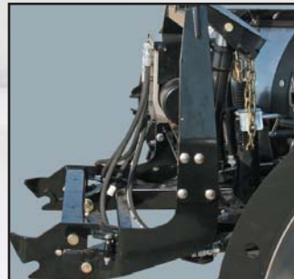
Contoured lift frame provides greater ground clearance
