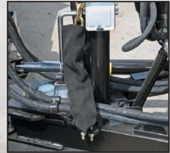
Adjustable/removable jack stand provides maximum flexibility for a wide range of mounting conditions & surfaces
