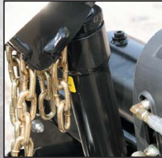
Lift arm w/heavy-duty 2" x 6" lift cylinder and 35° travel provides exceptional snow stacking
